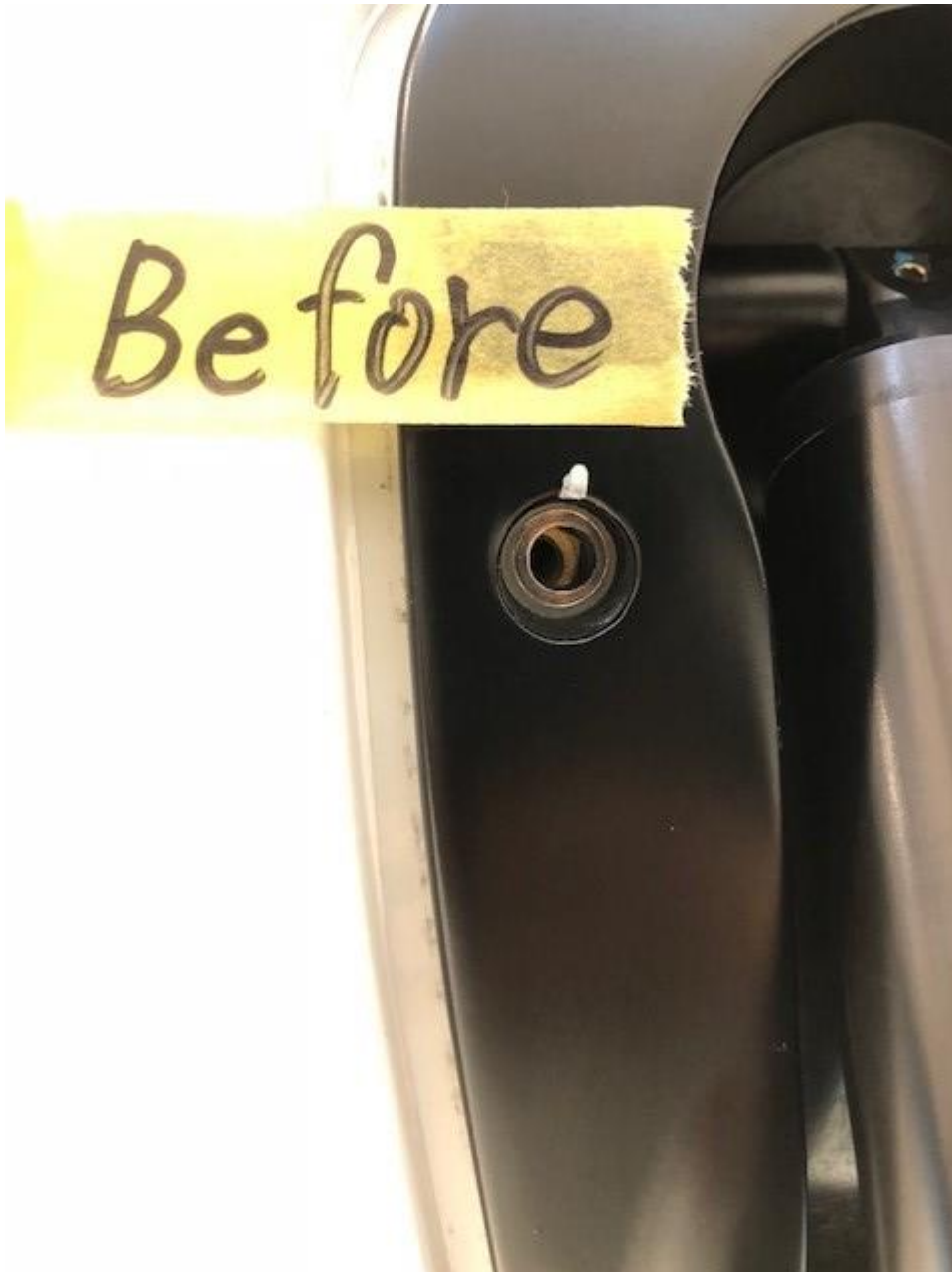
Figure 1: Airbrake panel holes not aligned.
